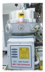
Low power consumption-vibration (LPV) sensing IC was settled on the IPX vacuum pump of Lam 2300 8" etcher for real time vibration analysis.
