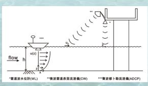
The Taiwan Typhoon and Flood Research Institute has developed the Automatic Real-time River Discharge Estimation Technique. With this technique, the river flow discharge can be estimated instantly, accurately and automatically
