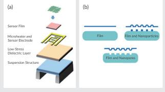
(a) Structure of the smart gas-sensing chip; (b) Nanotechnologies applied in the chip.
