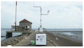
■ Southwest airflow observations with a Lidar wind profiler at Hanbou intertidal zone (Changhua coastal area)
