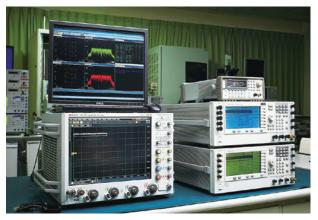
Millimeter wave multichannel transceiver measurement system
