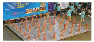
Nodels were tested on a shaking table
