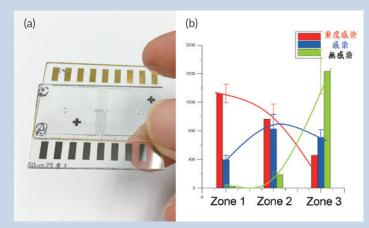
(a) Microfluidic chip for the rapid detection of dengue fever virus infection;
