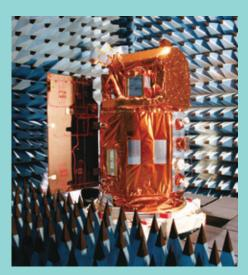
■ Electromagnetic compatibility test performed for the FORMOSAT-5 satellite
