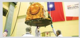
■ Assembling the FORMOSAT-5 satellite optical remote sensing instrument and spacecraft
