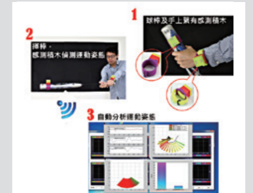
▲ A posture sensing system made from sensor building blocks
