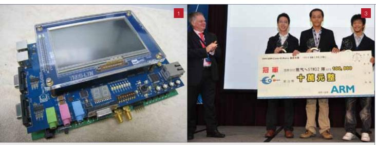
LCD touch panel module for video and audio multimedia applications & fieldprogrammable gate array (FPGA) core modules
