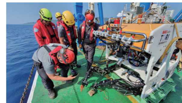
◀ 海洋中心與中山大學合作研發之輕型工作級 ROV Light Work-Class ROV developed by TORI and National Sun Yat-sen University
