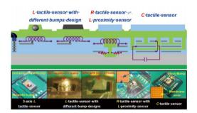
CMOS-MEMS tactile sensors
