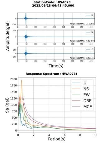
An example of acceleration waveforms and response spectra observed by a strong motion station
