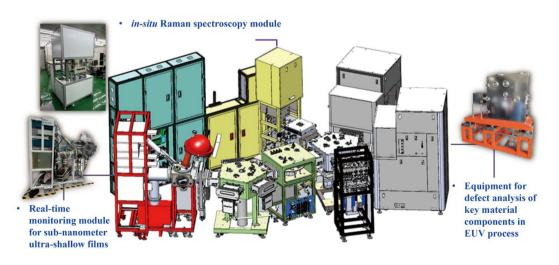
▲ On-site inspection equipment for cluster semiconductor process technology
