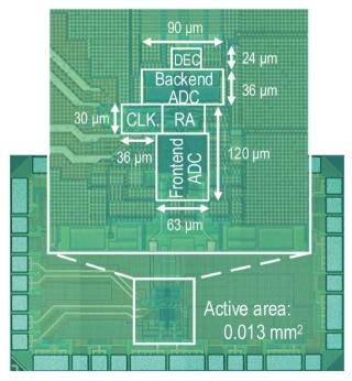
▲ High-resolution 130MSPS pipelined SAR ADC
