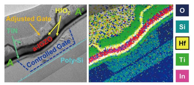
▲ Heterogeneous IGZO/poly-Si stacked complementary field-effect transistor structure
