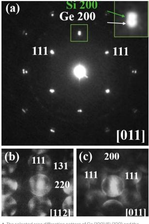
▲ The selected area diffraction pattern of Ge (100)/Si (100) and the converged beam electron diffraction patterns of (b) Ge (111) and (c) Ge (100)
