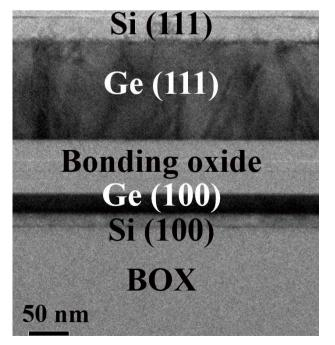
TEM of germanium substrates with different crystal orientations after bonding
