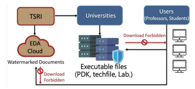
NI6 ADFP information security structure with unidirectionality to ensure security of sensitive process data
